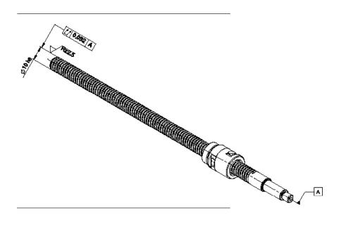
The changeover to a screw outside diameter of Ø10 for ball screws with nominal Ø10 is an important change that is beneficial for you as a customer, but also for us as a manufacturer.
